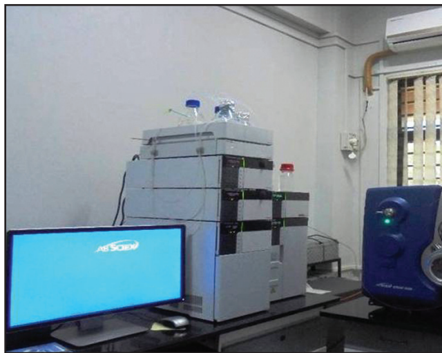
Highly sensitive LC-MS/MS system (Qtrap 4500, ABSciex, USA)
